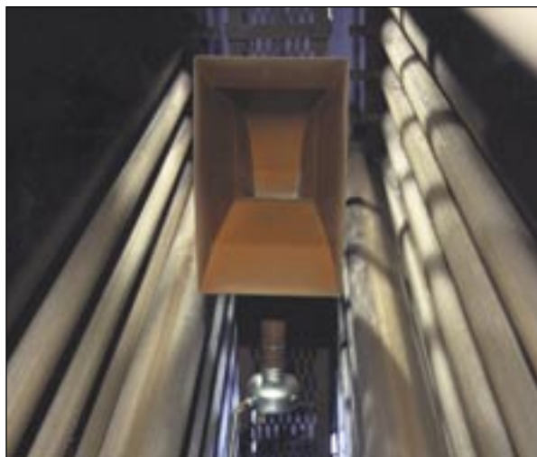
Fig. 7. Powerwave® acoustic horns can be chain-hung inside baghouses to provide effective cleaning of filters, without the abrasion and flexing.
