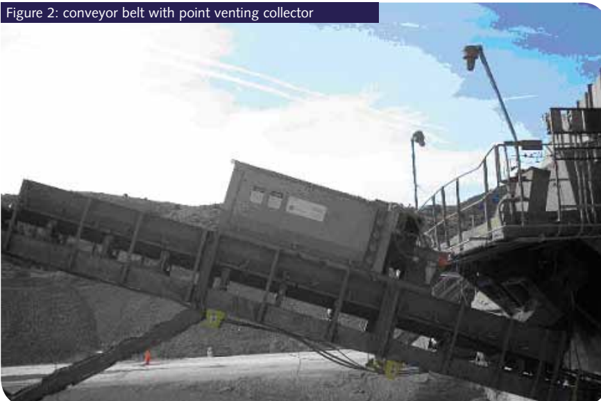
Figure 2: conveyor belt with point venting collector
