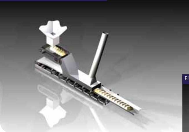
Figure 3: typical belt venting design
