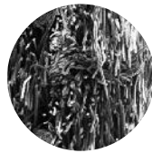
Side view of standard polyester magnified 50 times.
