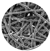
Face view of spunbond polyester magnified 100 times.
