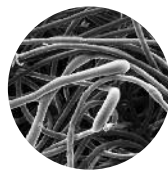
Face view of standard polyester magnified 100 times.
